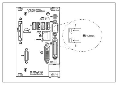
Figure 3-4. Ethernet Connector Location and Pinout
